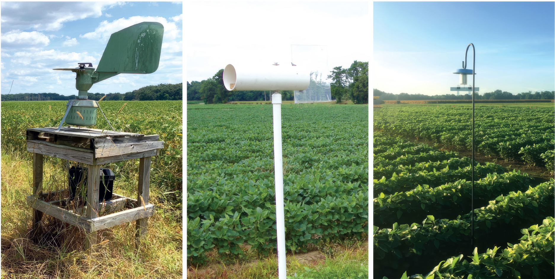
Spore traps placed around soybean fields in Louisiana include the Burkard spore trap (left), wind vane spore trap (center) and garden motor spore trap. These are used to monitor peaks of spores of the pathogens causing Cercospora leaf blight of soybean. Photos by Sara Thomas-Sharma
